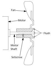
Figure 7 - Fan Cross Section
